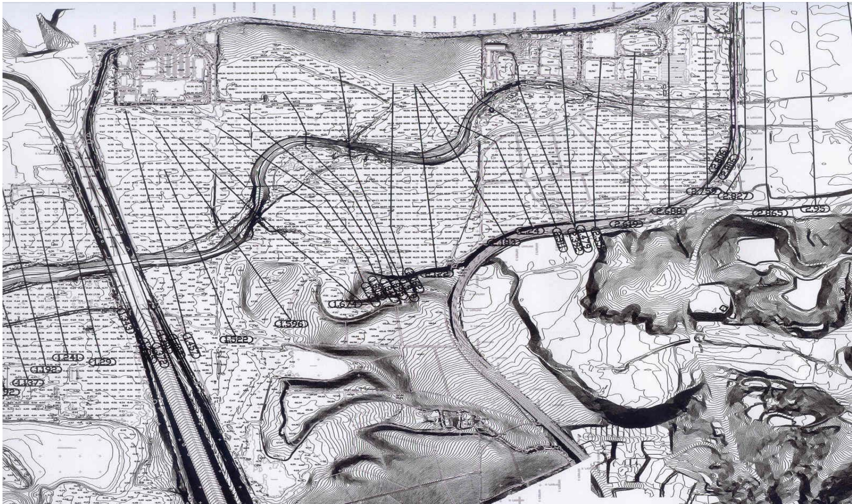
Figure 2.25. Lower San Dieguito River Hydraulic Modeling Cross Sections
