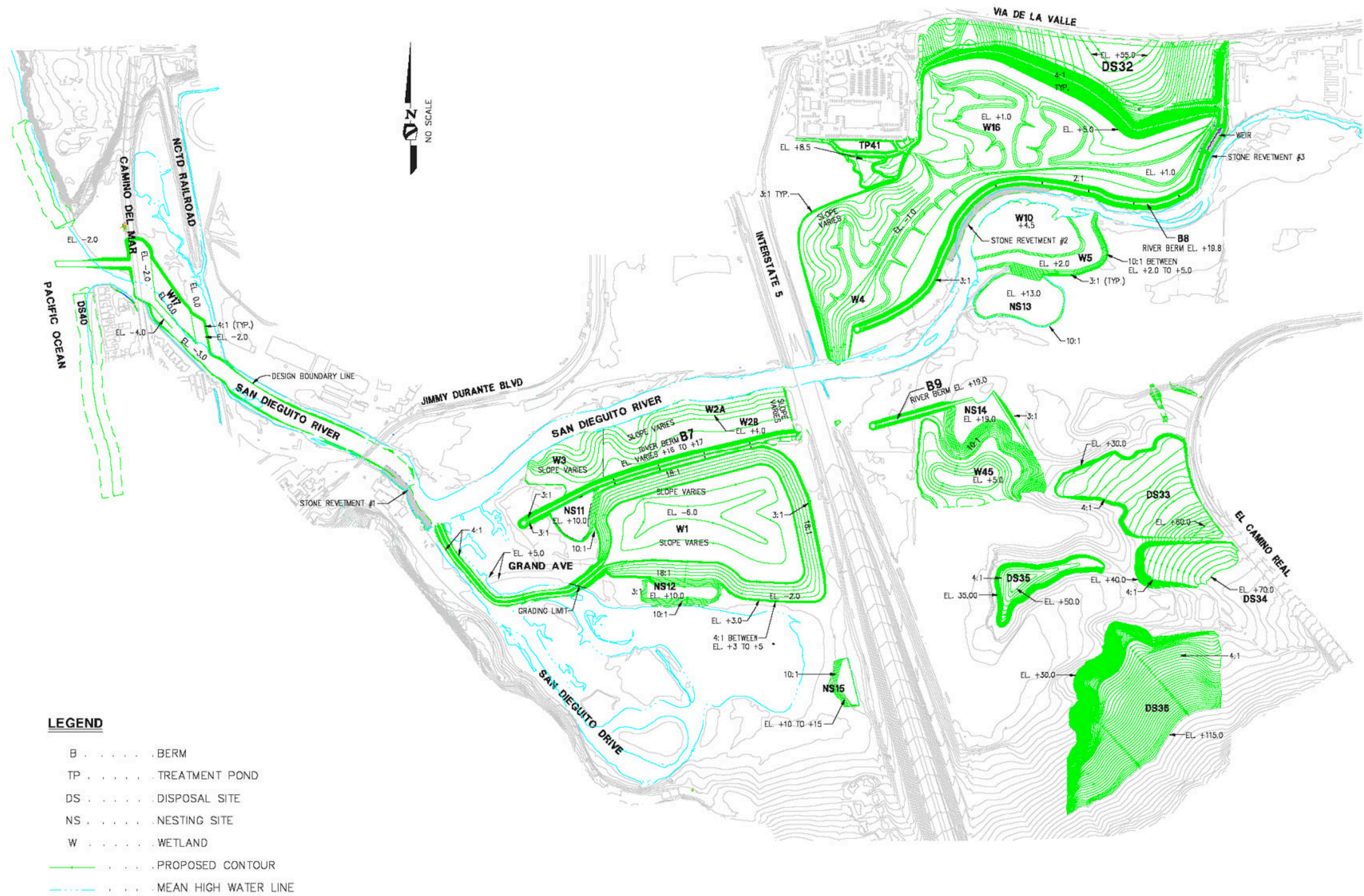
Figure 4.2. San Dieguito Wetlands Restoration Project - Grading Plan
