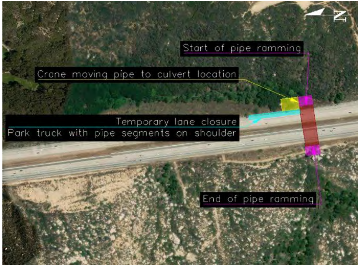
Figure 6.9. Construction Stage Two - Corrugated Steel Pipe.
