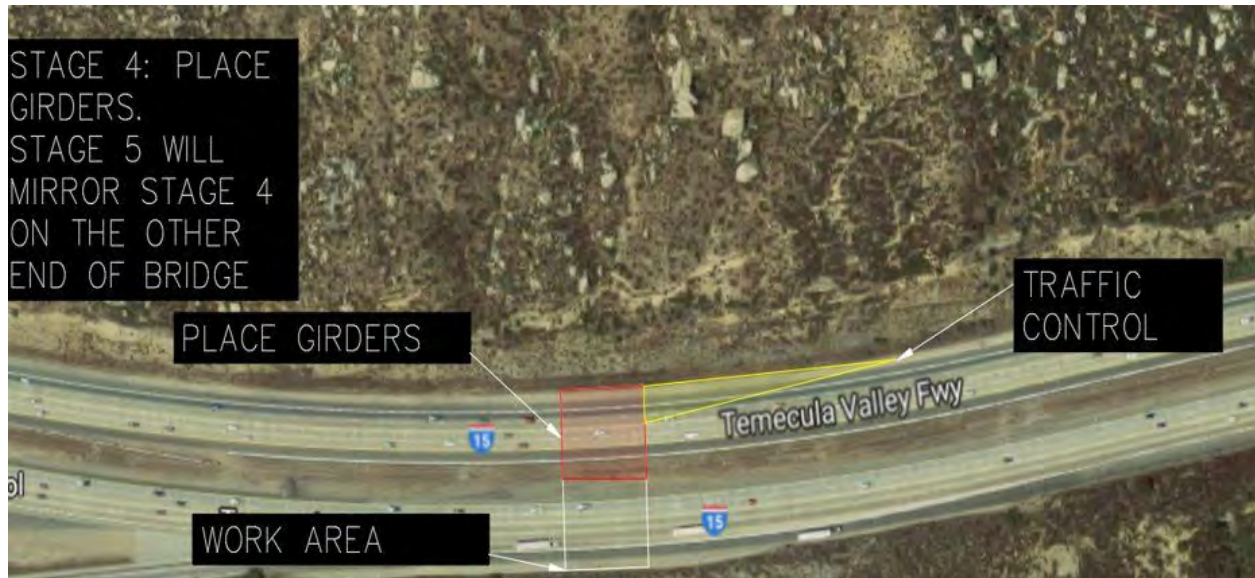
Figure 5.12. Construction Stages Four and Five.
