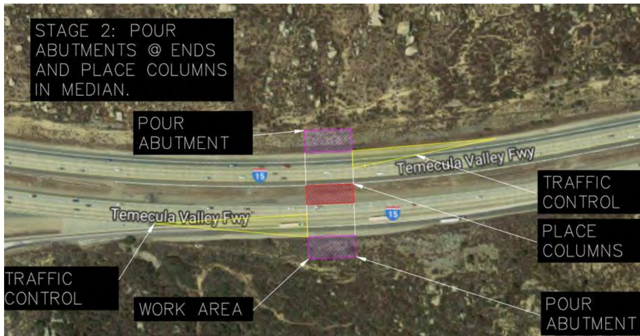
Figure 5.10. Construction Stage Two.
