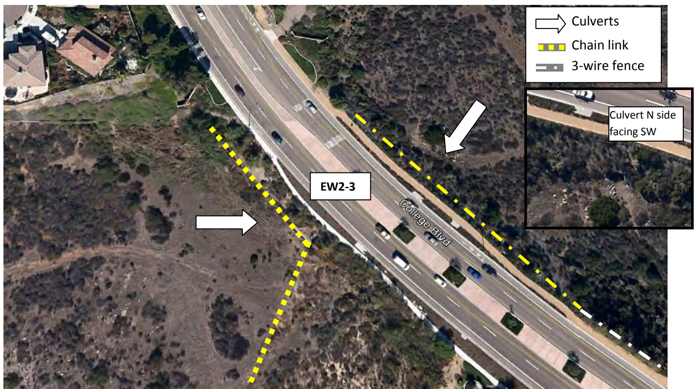
EW2-3, High priority. College Blvd. and Robertson Ranch East Preserve. Undercrossing. Fencing on north side is 3-wire and will allow for wildlife to move up and over the road. A portion of the southern side is fenced with chainlink. Animals
